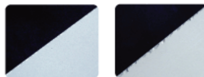
Comparison of Alpha Libero-100 (left) and typical natural stone cutting blade used on Limix
